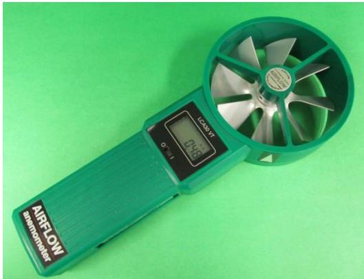
Figure 5-15: A hand-held anemometer for measuring air velocities
